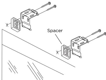
Spacers are available for use on windows with a projected molding. They are  $\frac{3}{8}$ " thick and allow the shade to be mounted flush with the outside edge of any standard window molding. They are available by contacting our Customer Care Department at 800-800-3329.
