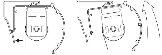
**TO REMOVE:** To remove the shade use a flathead screw driver and gently pry the bracket release tab between the bracket and the headrail in the back of the shade headrail. Repeat this for each bracket until the shade is free from the mounting brackets. Use Caution and support the shade while releasing it from the brackets so that the shade does no fall.
