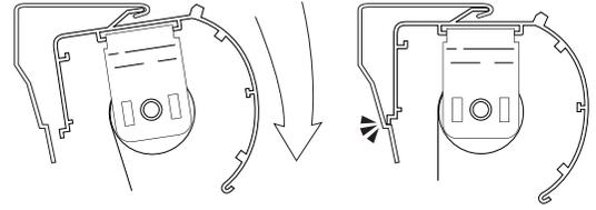
TO INSTALL: Hook the front top lip of the bracket into the channel on top of the rail. Rotate the back of the shade upward until the back of the rail engages into the bracket.
