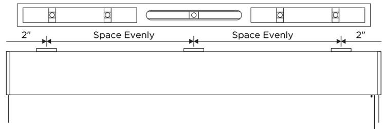
NOTE: Measure and mark all bracket locations before installing.
