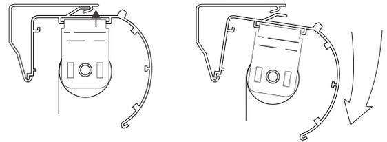
**TO REMOVE:** To remove the shade use a flathead screw driver and gently pry the bracket release tab between the bracket and the headrail on the top of the shade headrail. Repeat this for each bracket until the shade is free from the mounting brackets. Use Caution and support the shade while releasing it from the brackets so that the shade does no fall.
