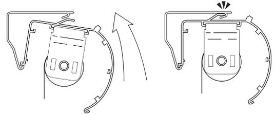
TO INSTALL: Hook the back of the rail onto the tab on the bottom of the bracket. Rotate the front of the rail upwards until the rail engages into the brackets.
