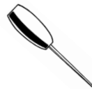
Awl (or tool for starting a screw hole)
