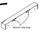
Position the bottom rail stop so it does not interfere with the mounting brackets.
