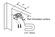
• The Brackets should be installed at each end, with the centerline of the brackets positioned 2" from the ends.
