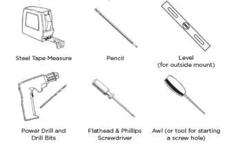
Included in your order is all the hardware necessary for a normal installation. Depending on the mounting surface, fasteners other than the screws provided may be required. Wall board and plaster require the use of anchors such as expansion or toggle bolts. Bricks, tile and stone need special plugs and drill bits. Wood should always be pre-drilled to avoid splitting.
