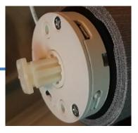
Power switch (If motor is not responding check this switch) I = Motor on 0 = Motor off
