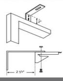
Optional Extension Brackets are used to project the back of the shading up to 2 1 /2" from the mounting surface.
