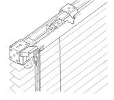
While supporting the bottom of the blind, unwind the draw cords and gently lower the blind to its full length. (See "Blind Operation", Page 8)
