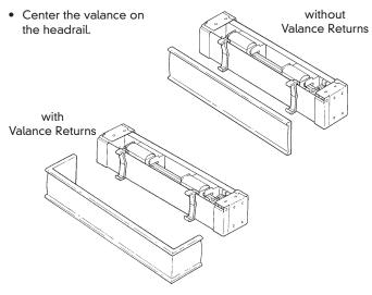
• Insert the top edge of the valance into the top lip of the Valance Clips. Using a downward rolling motion, gently push the bottom edge of the valance into the Valance Clips until you hear the valance "snap" into place.
