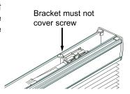
Using the Installation Bracket as a template, measure to the edge of the bracket and mark the hole locations with a pencil for drilling.
