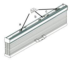
The center of the right end bracket must be placed 1" to 2" from the end, so that it does not interfere with the transmission screw.
