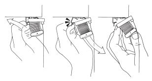
• Rotate the back of the headrail down and carefully lift the headrail off of the front hooks of the mounting brackets.
