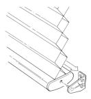
• Lower the shade and flex the hold down bracket outward so that the pin can be inserted into the hole in the end cap.
