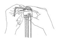
To remove the headrail, push up on the tail of each mounting clip to release the headrail from the brackets.
