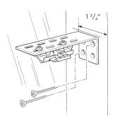
• Recess the back of the bracket no more than  $1\frac{3}{4}$  from the front edge of the window casing.
