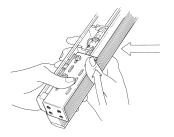
• Remove the mounting brackets from the headrail by pushing the back of the bracket forward and up with your thumb.
