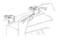
• Mount each bracket making sure all brackets are installed level and in line with each other.
