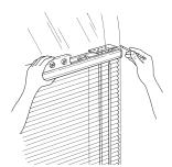
• Once the blind is level, mark the wall or molding on the top edge of each mounting bracket.
