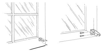
• Mount the hold down to the side or back of the window frame so that the pin lines up with the front hole in the ottom rail end cap with the blind fully lowered.
