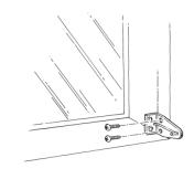
• Mount the hold down to the side or back of the window frame so that the pin lines up with the front hole in the ottom rail end cap with the blind fully lowered.
