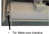
Tip: Make sure charging port is pointing down and accessible to plug in micro USB charging wire.
