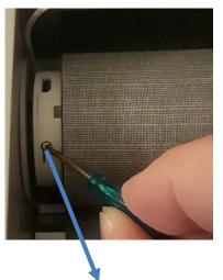
P1 button (Remote will come with small blue screw driver that can be used to push the P1 button)
