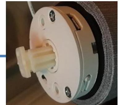
Power switch (If motor is not responding check this switch)
