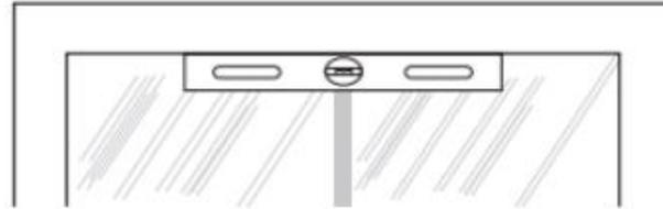
**WARNING:** If the headrail does not sit level, the Window Shading will not roll up evenly. This could damage the edges of your shading! Your Window Shading has been leveled and weighted in our factory. Shims have been provided to allow you to compensate for uneven mounting surfaces and ensure balanced operation.
