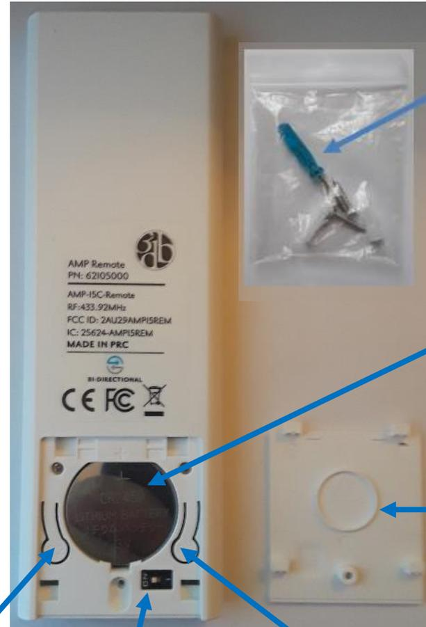
**Small Blue Screw Driver** – Used to secure back cover on remote. **Also can be used to press the P1 button. LEAVE W/CLIENT**
