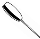
Awl (or tool for starting a screw hole)
