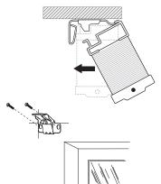
Remove the mounting brackets from the headrail by pushing back and up on the "tail" of the bracket.
