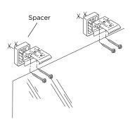
Spacers are available for use on windows with a projected molding. They are  $\frac{3}{8}$ " thick and allow the shade to be mounted flush with the outside edge of any standard window molding. They are available by contacting our Customer Care Department at 800-800-3329.
