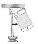
Remove bracket by using a flat head screw driverand push up between racket and head rail.
