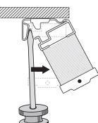
• Rotate the back of the headrail down and carefully lift the headrail off of the front hooks of the mounting brackets.
