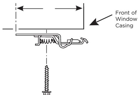
The back of the bracket must not be mounted any further back than 1 3/4" from the front of the window casing. The front of the bracket will extend slightly beyond the front of the window casing when installed correctly. Templates have been provided to assist with placement of the brackets.
