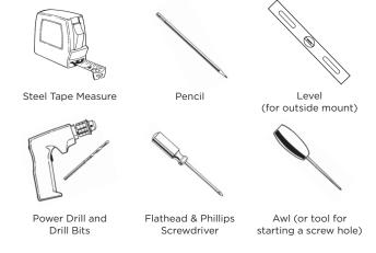
Included in your order is all the hardware necessary for a normal installation. Depending on the mounting surface, fasteners other than the screws provided may be required. Wall board and plaster require the use of anchors such as expansion or toggle bolts. Bricks, tile and stone need special plugs and drill bits. Wood should always be pre-drilled to avoid splitting.
