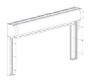
Slide the channels all the way up until they touch the bottom of the cassette. Hold a level on the siderails and adjust until it is level vertically. Then fasten with screws in the pre-drilled holes.
