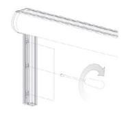
• Use a flat head screw driver and rotate the locks clockwise to secure the side guides together.
