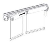
• Insert the second shade into the center link bracket and clip the idler into the idler bracket.
