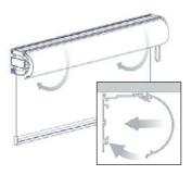
• Insert the round or square cover onto the cassette back and rotate it down to clip into position.
