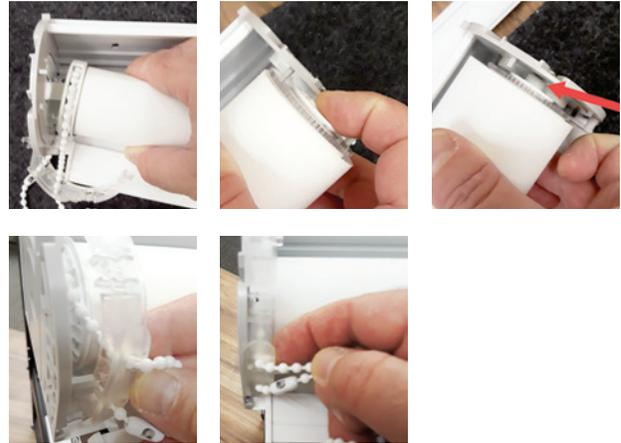
Once you have the shade back into the Cassette now it is time to reattach the Fascia. The Fascia sits in a groove on top of the Cassette and snaps into the end plates on the right and left side. Insert the Round or Square fascia onto the Cassette back groove & rotate down to clip into position on the right and left side, you will hear it snap into place.
