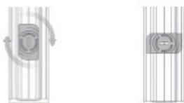
Unlocked Position: rotate clockwise to lock      Locked Position
